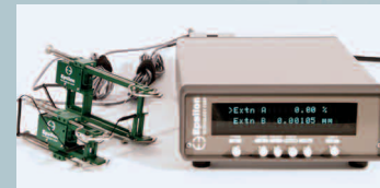
Model DSM-Plus two channel high accuracy strain meter with Model 3542
