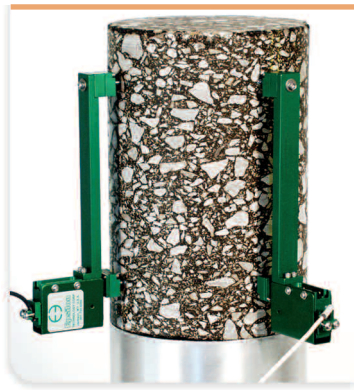
Model 3909-0400 with 4 inch gauge length
