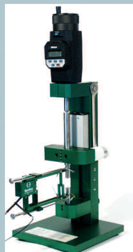
Model 3590 with Model 3542 axial extensometer
