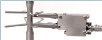
Model 3555 with 0.5 inch gauge length and +10/-5% measuring range
