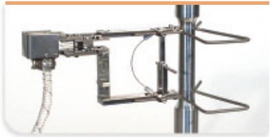
Model 3555BP with 50 mm gauge length and +20/-10% measuring range
