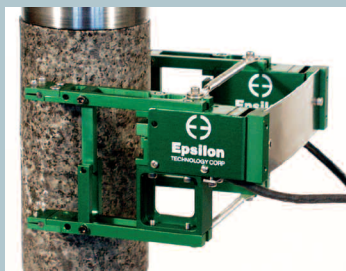
Model 3542RA1 extensometer with 50MM gauge length
